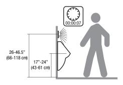
With urinal flush controls a minimum distance of 36" (90 cm) to the opposite wall must be observed to ensure problem-free detection. If urinal flush controls are mounted on opposite walls, a distance of 60" (150 cm) must be observed. Urinal flush controls mounted next to one another must be at least 20" (50 cm) apart.
