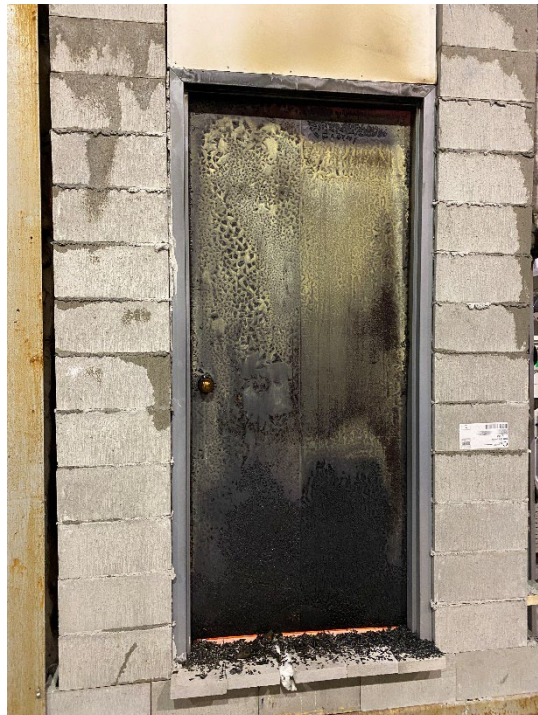
Figure 9: The unexposed side of assembly 1 32 minutes into the fire test.
