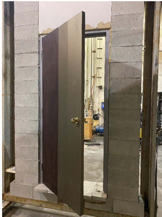
Figure 7: The latch edge of assembly 1 prior to the fire test.
