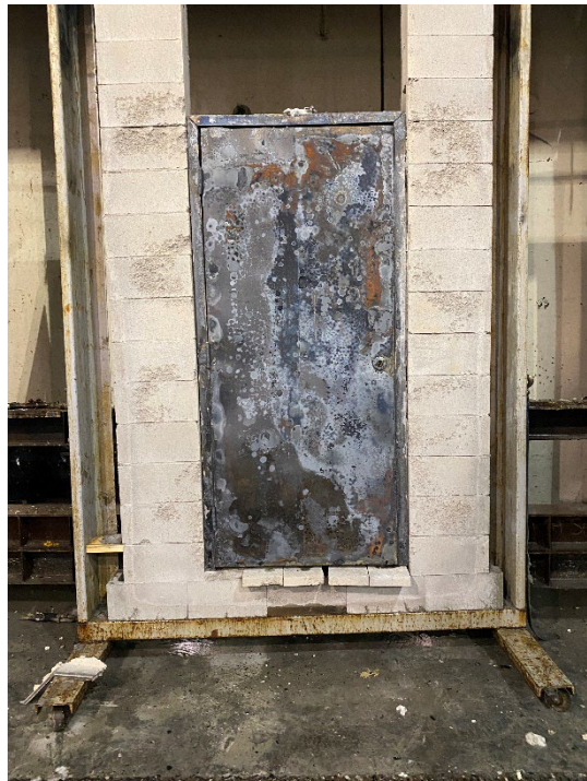
Figure 11: The exposed side of assembly 1 after the hose stream test.
