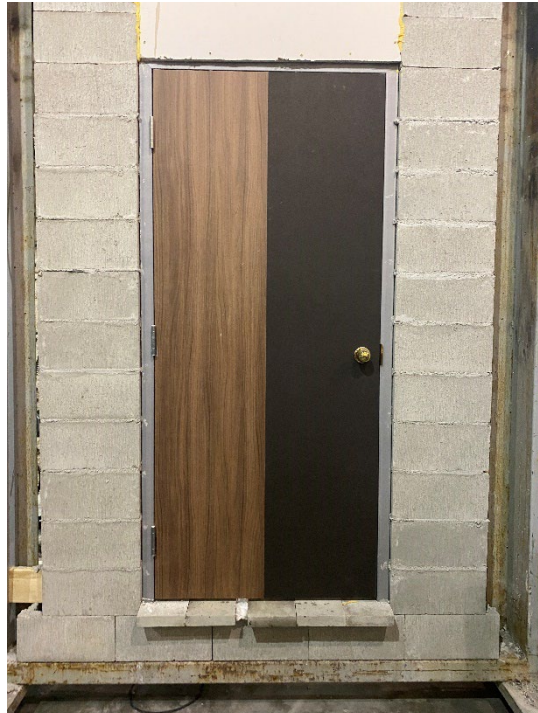
Figure 12: The exposed side of assembly 2 prior to the fire test.
