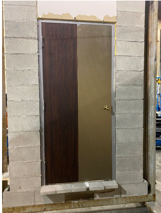
Figure 6: The exposed side of assembly 1 prior to the fire test.
