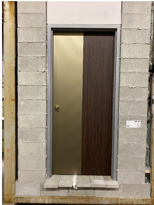
Figure 8: The unexposed side of assembly 1 prior to the fire test.
