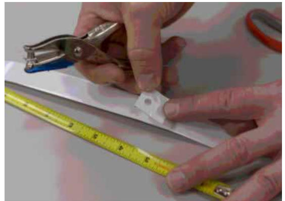
Figure 2. Preparing the test strips
