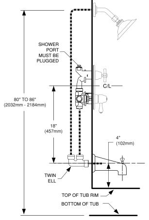
IMPORTANT: WHEN NOT USING A DIVERTER SPOUT A SEPARATE DIVERTER VALVE MUST BE USED.
