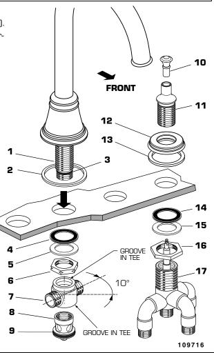
Insert FIBER WASHERS (1) into COUPLING NUTS (2) onto threads of T-PIECE and tighten.
