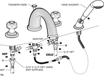
IMPORTANT: It is strongly recommended that access be provided for all enclosed mechanical parts to this system.
